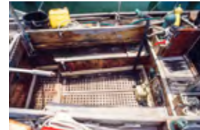
Here's the original cockpit; too deep, too uncomfortable and far too many places for it to leak. That Whale Gusher 25 pump got a lot of use!
