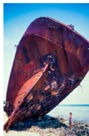
The County of Roxburgh was wrecked in 1906. It's interesting to note the difference in corrosion of the iron plating between the seaward and landward sides. There's a fascinating website about the ship at www.county-of-roxburgh.com/
