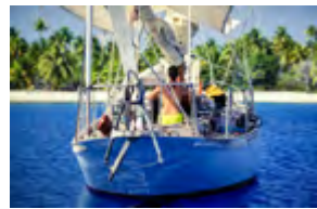
A sun awning keeps the deck and interior cool although a wind scoop on the forehatch makes the biggest difference. The Aries self-steering gear on the stern is arguably the most important gear on the boat. Originally made by Nick Franklin in the UK, then in Denmark and now in Holland. If I were to ever have another yacht, I think this is what I would buy first.
