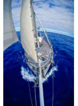
Fisheye lens view from the bowsprit with the 45lb CQR bower anchor and the 50lb fisherman anchor ready to deploy.
