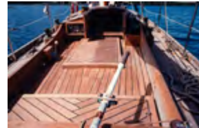
I finally replaced the cockpit in Whangarei, leaving the existing cockpit coamings in place. The two hatches are for removing the engine and for a watertight locker for petrol and kerosene. A big double bed was beneath the new cockpit. This alteration improved the quality of life aboard immeasurably.
