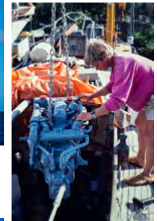
Installing the newly painted Perkins 4.108 engine while there is still a big hole where the cockpit used to be. I built the new cockpit while Eila was afloat in the Town Basin in Whangarei, New Zealand.
