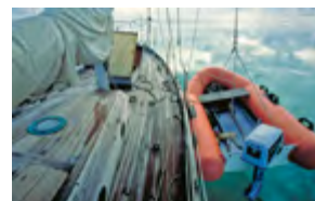
Anchored in the calm at Fanning Island we lift the dinghy out of the water with a halyard to reduce fouling on the bottom. You can see the wind chute (or scoop) which normally would be funneling the breeze down below.
