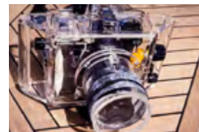
The housing I built for the Canon F1n and Speedfinder. I had the remote sensor for a Vivitar flash gun wired into the camera housing.
