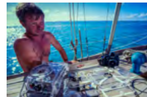
Testing a new mini dome off Moorea, fortunately without the camera in the housing, the back collapsed, so I surfaced with about 20 pieces stuffed in my wetsuit. I had Tensol 70 glue aboard and was able to buy 12mm Perspex in Papeete. A week later I had repaired the housing by replacing the top plate and making a better designed, much stronger back.
